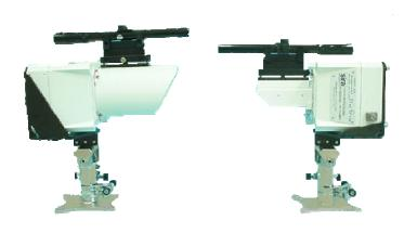
SafEye 200 Series Open Path Gas Detector is a self-contained, fast response optical gas detection system. It detects combustible gases at concentrations lower than the explosion limit (LEL) over a "Line of Sight" of up to 460 ft. (140 m) long. SafEye is the preferred system for offshore oil companies because it is immune to false alarms caused by partial blockage and extreme weather conditions (fog, rain, snow) and direct or reflected sunlight, flame and other black body radiation sources.
